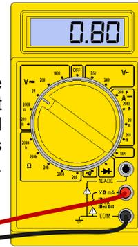
Voltage Should Be Between 0.8 and 4.3 Volts
