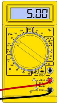
Voltage Should Be Between 4.3 and 5 Volts
