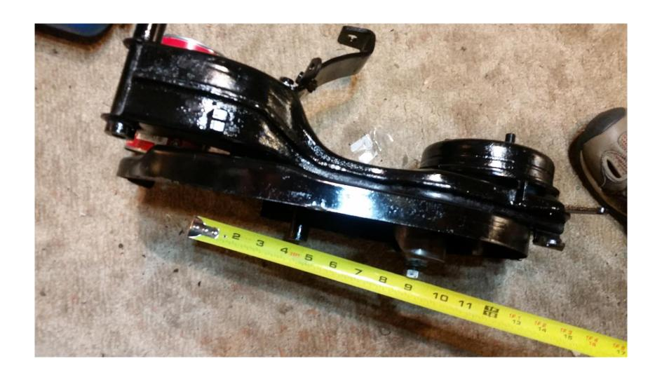
2&1/4 "from engine mount face to sprocket mount face (engine shaft would need to be 3 inches long)
