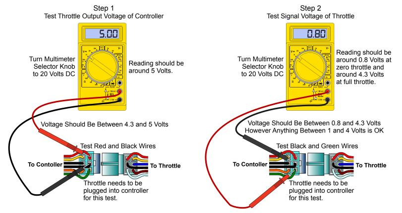
If the controller does not have a 4.3 through 5 Volt output to the throttle then the controller or one of the parts connected to it such as the power switch, fuse or circuit breaker, wiring harness, connectors, brake switch, or battery pack is faulty.
