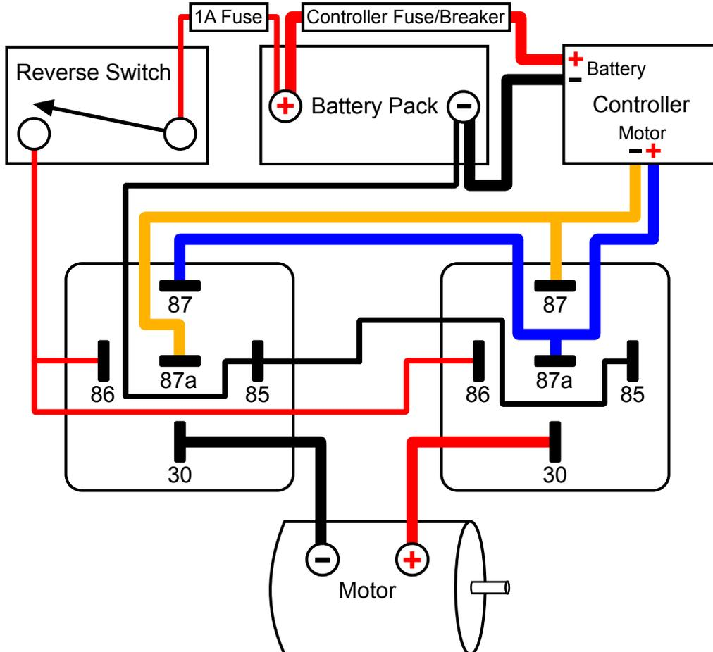
22 gauge (AWG) or thicker wire is suitable for the switch and relay coil wiring.
