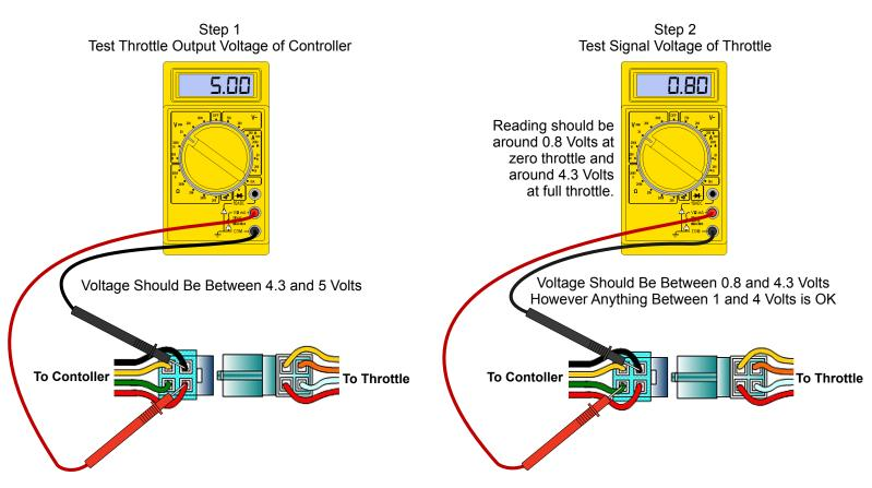
If the controller does not have a 4.3 through 5 Volt output to the throttle then the controller or one of the parts connected to it such as the power switch, fuse or circuit breaker, wiring harness, connectors, brake switch, or battery pack is faulty.
