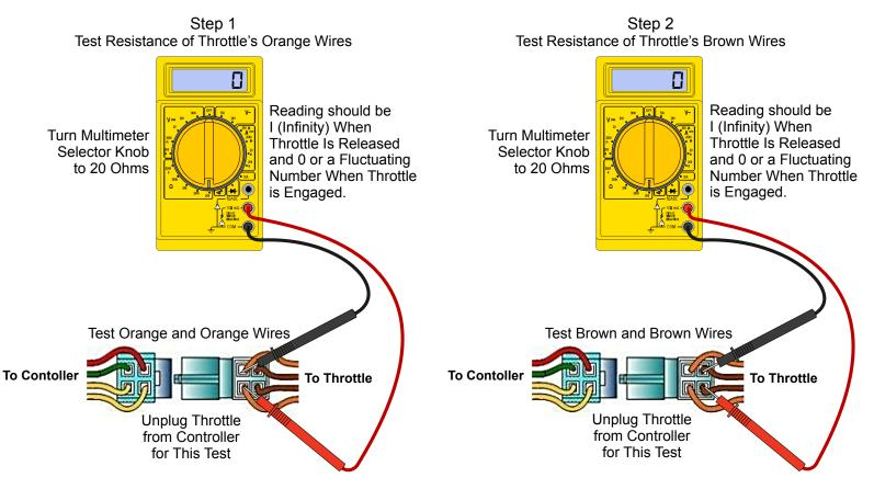
If the resistance between both the two orange wires and the two brown wires changes from I (Infinity) to 0 (Zero) (or a fluctuating number) when the throttle is engaged then the throttle has passed the test and is good.
