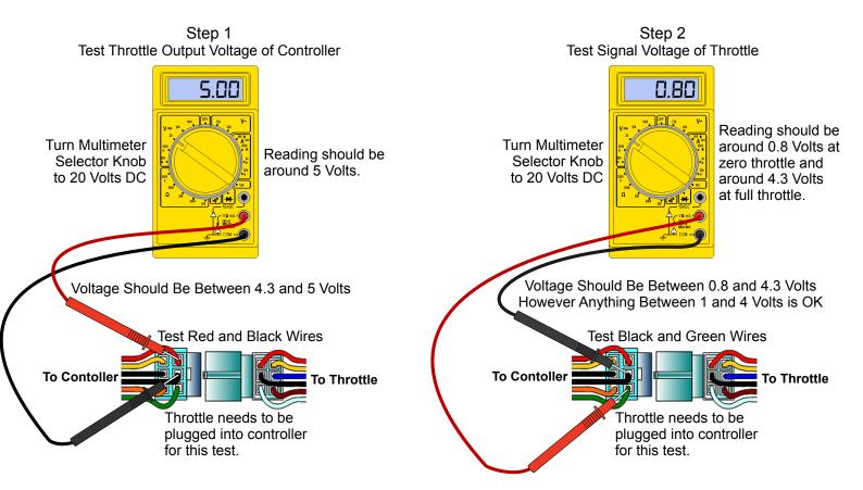
If the controller does not have a 4.3 through 5 Volt output to the throttle then the controller or one of the parts connected to it such as the power switch, fuse or circuit breaker, wiring harness, connectors, brake switch, or battery pack is faulty.
